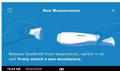
1. Ensure that your handheld is switched on and connected to the basestation (the bluetooth symbol on the handheld finished blinking, the **handheld connected** icon is shown).
