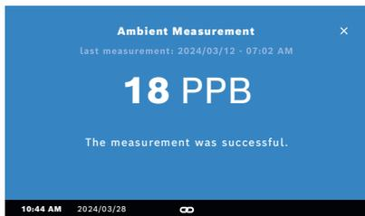
Ambient NO measurement may help to interpret FeNO measurement results. To perform an ambient NO measurement:
