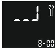
1. The **wrench** symbol on the handheld and the basestation indicates that the reconditioning process is on going. The remaining reconditioning time is shown in minutes.
